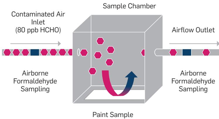
Schematic of a small-scale testing chamber to monitor formaldehyde scavenging performance of a coating.
